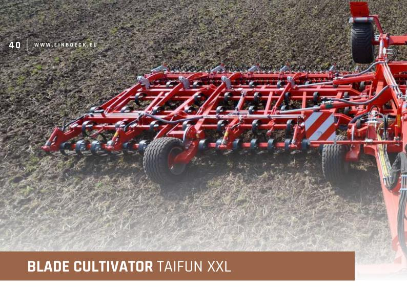
The blade cultivator TAIFUN is a multi-purpose, highly efficient machine. It is a classic machine for seedbed preparation due to its high and spacious frame construction – especially for areas with catch crops and winter greening. The incorporation of liquid manure and organic fertilizer, as well as light and shallow stubble turning or second stubble cultivation and the combat of couch grass are ideal jobs for the TAIFUN.
