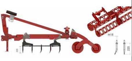
G-2FZ: mini seedbed tine section + flat rod crumbler Ø 380 mm / 14.96" + serrated crumbler Ø 320 mm / 14.96" Mini seedbed tine section with spring tines, 5-rows, firmly mounted, height adjustable + big flat rod- and serrated crumbler for light to sandy soils, flat rod crumbler ensures high load capacity
