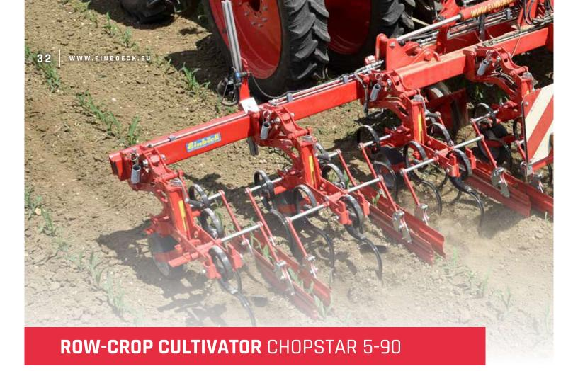
The CHOPSTAR 5-90 has up to 5 times per hoeing element and is used in row-crops with up to 90 cm / 35.40" row spacing, such as corn, sunflowers, etc. Depending on the conditions and the aim of the hoeing pass, a variety of tools such as heaping elements, heaping sweeps, weeder tines mounted behind the elements, finger weeders etc. can be attached to the front or rear implement.
