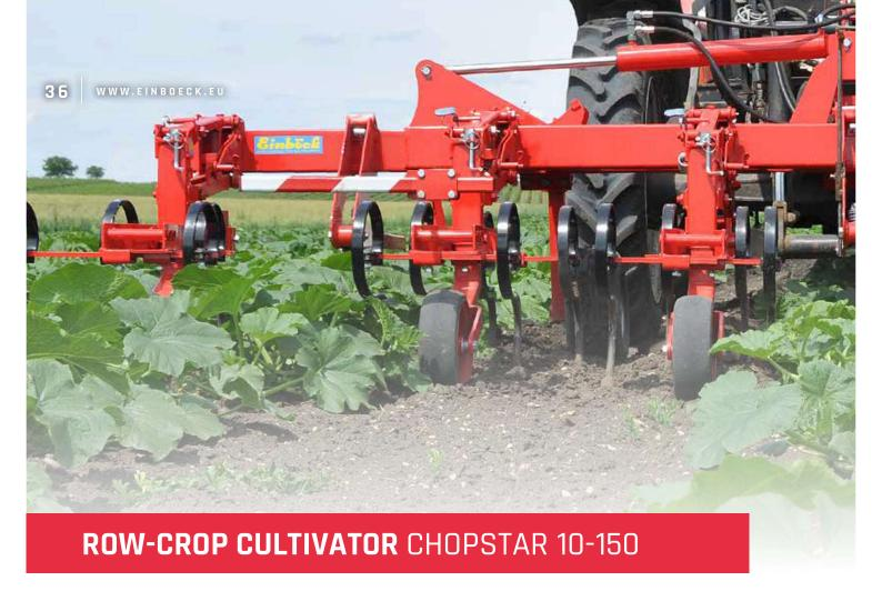
The CHOPSTAR 10-150 has two hoeing elements per row and up to 10 tines and can be used in row-crops with a row distance of up to 150 cm / 59", such as pumpkin, etc. Depending on the conditions and the aim of the hoeing pass, a variety of tools can be attached to the front or rear implement, such as heaping elements, heaping sweeps, weeder tines mounted behind the element, finger weeders, etc.
