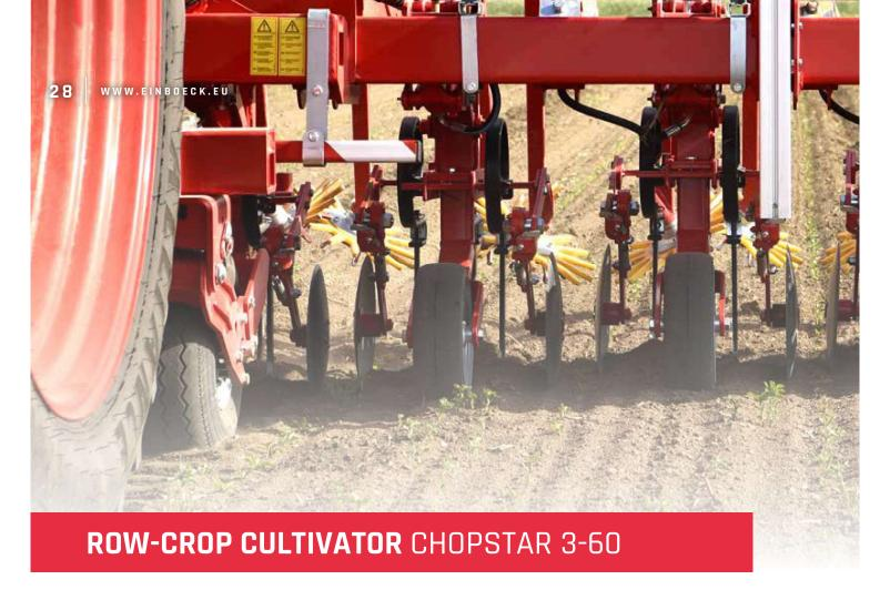
The CHOPSTAR 3-60 has up to 3 tines per hoeing element and can be used in row-crops with a row spacing of up to 60 cm / 23.60" (such as beets, soybeans, field beans, etc.). Depending on the conditions and the aim of the hoeing pass, a wide range of tools such as heaping elements, heaping sweeps, trailed weeder tines, finger weeders, etc. can be attached to the front or rear hoeing machine.
