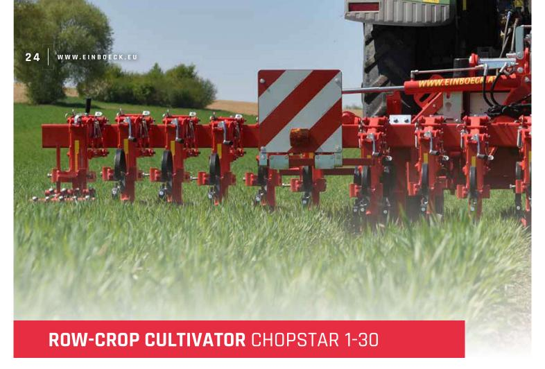
The CHOPSTAR 1-30 has 1 tine per hoeing element and can be used in row-crops with a row spacing of up to 30 cm / 11.80", e.g. cereals, field beans, lupins, etc. Depending on the conditions and the aim of the hoeing pass, weeder tines mounted behind the element or different sweeps (such as ultra-flat) can be mounted on the front or rear hoeing machine.
