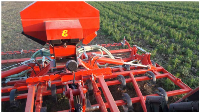
Seedbed combination with duckfoot sweeps (working depth 5 cm / 2"), cuts through the entire surface and destroys the cover crop. ATTENTION: soil should not be sensitive in respect of silting
