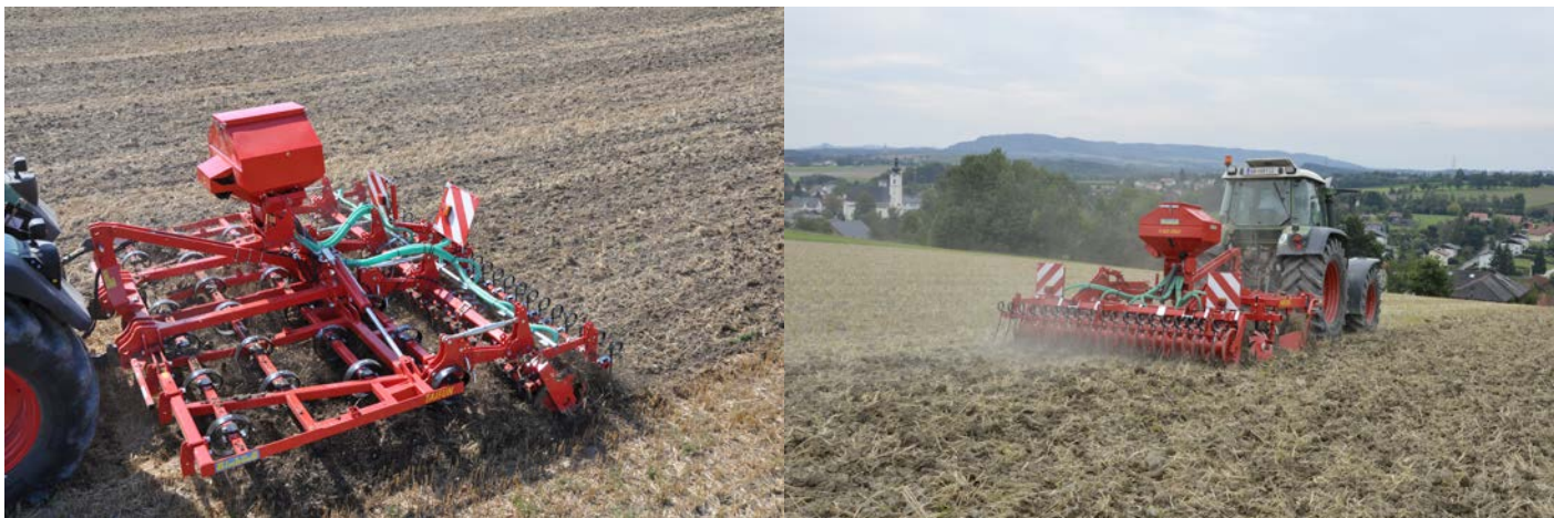
The picture on the left shows a shallow stubble cultivation pass (working depth approx. 5 cm / 2"), the picture on the right shows the second stubble cultivation (working depth approx. 10 cm / 4") in combination with planting a cover crop.
