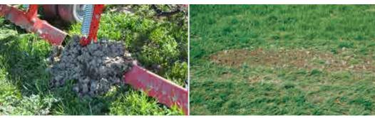
The **triangular front levelling plate** of the PRO-series.
