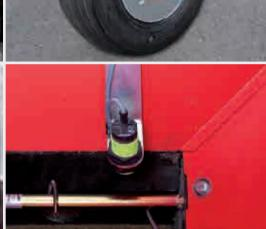
The **tank level sensor** signalizes, when the tank is getting empty. The sensor works inductively, therefore it is vibration independent.
