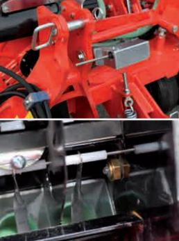
The sensors of the **airflow monitoring** signalize, whether one or more seeding hoses are clogged (optional).
