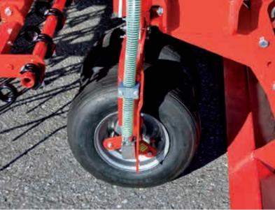
**Ground drive** via the support wheel (PNEUMATICSTAR). The flexible shaft, which runs a infinitely variable oil bath gearbox, is protected by a hose. The information about working speed is provided from the support wheel. There is no additional ground wheel necessary.
