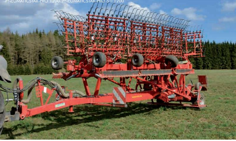
The sophisticated **retraction mechanism** together with putting the tines into the lowest angle position makes it possible to reduce the transport width to only 3 m
